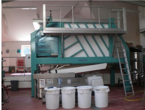
**Figure 2.23:** Grape processing equipment representing a high kW power rating but relatively low kWh energy usage
