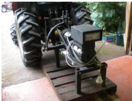
Figure 2.11: Examples of power take off generator coupled to a tractor in an English winery
