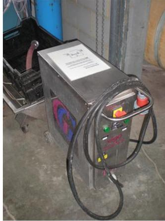
**Figure 2.67:** Electrical ‘resistance’ steam generator
