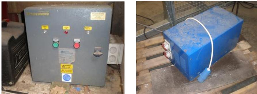
Figure 2.10: Examples of phase converters used in English wineries
