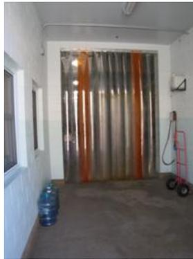
**Figure 2.35:** Use of strip curtains to reduce unwanted air movement through an open door
