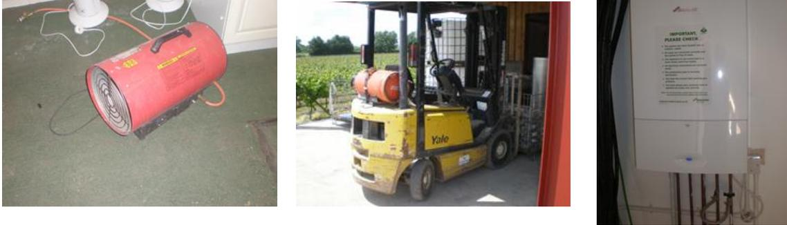
Figure 2.8: Examples of gas fuel usage in the winery (gas fired portable heater; gas fork truck, domestic hot water)
