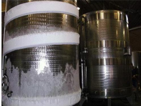
**Figure 2.48:** Cold stabilisation with external frozen condensation on exposed heat exchanger surfaces
